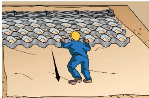
4. Expand sections down the slope.
