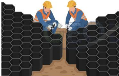
6. Connect sections side-to-side and end-to end.
