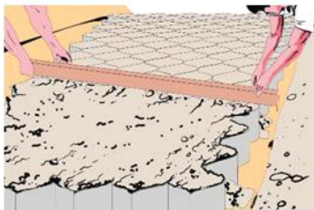
9. Remove excess material to expose top cell walls.
