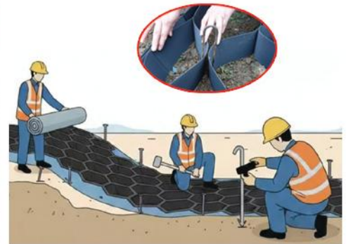
7. Hold sections open (use J-pins or Anchors or Wood stakes).
